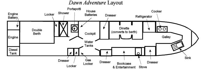
She is fitted with a Lombardini diesel engine (about 300 hours since new), an Enfield 130 Z-drive (about 160 hours since professional rebuild), and an 8 x 13 inch propeller. We have found this installation satisfactory on both canals and the River Weaver. Typical of GRP cruisers, she will travel at maximum allowable canal speeds with modest wake. For planning purposes, I estimate fuel consumption at 1 liter per hour, but this will vary depending on time spent in locks, battery charging, etc.
