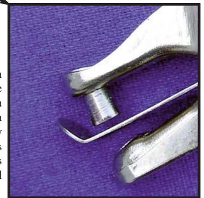
Figure 5. This photo of a cheap hand-punch shows the conical shape desired on a swinging arm. On such a design the punch actually rotates as it enters and leaves the die, and the taper allows both smooth motion and reduced clearance.
