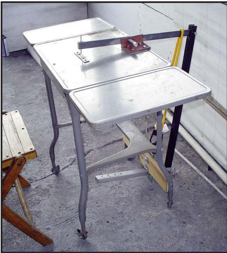
Figure 1. This shows the overall configuration of my punch. Pressure on the foot treadle is transmitted to the punch rocker by a steel push-tube. Most of the return force is provided by the weight of the push-tube, but a loop of shock cord provides a bit more "omph." I usually punch with the side extensions down, but use the extensions for trimming and stapling.
