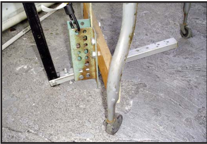
Figure 3. The treadle is made from a 15 inch piece of 3/4 inch by 1 1/4 inch steel channel. The pivot is located four inches from the rear end. The vertical bolt through the treadle provides an adjustable down-stroke stop.
