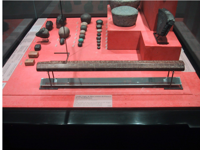
Figure 2. A cubit rule with graduated markings and other Egyptian standards in the Louvre.
