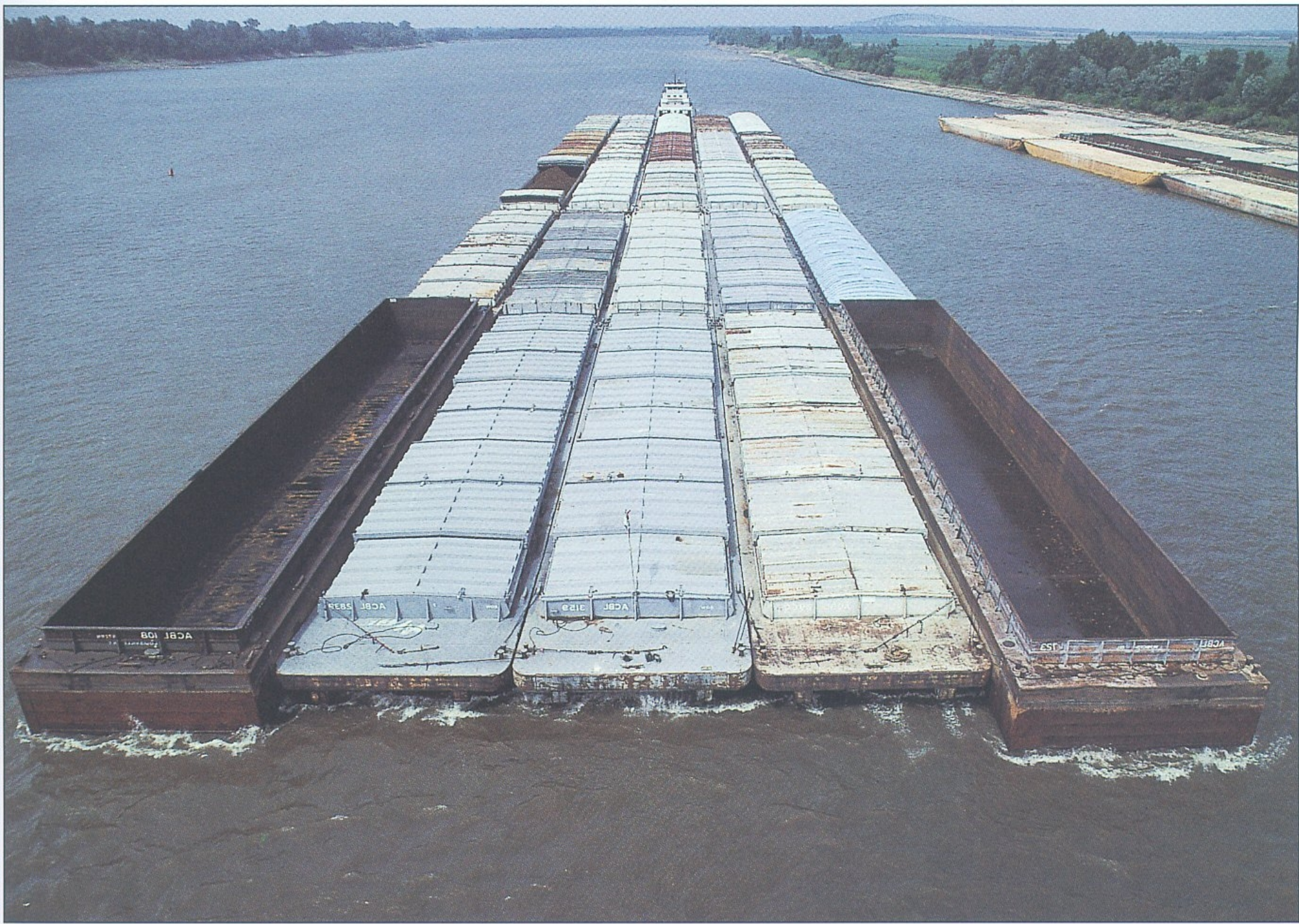
The U.S inland waterways system provides channel dimensions which enable users to deploy the most economical fleet of the largest pushed tows in the world. A tow of 40 barges with 60,000 tons (above) moves down the Lower Mississippi River.
